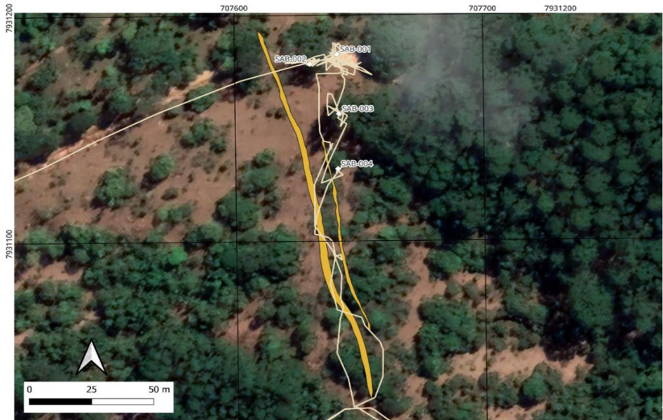
Figure 18 – Map of geological points at North Eucalipto Target. The Yellow line, the projection of the Iron Ore occurrence, and in white the geological points.
