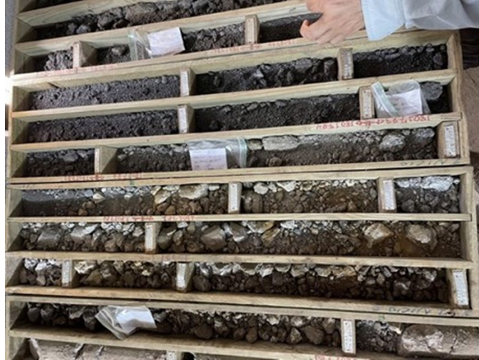
Figure 32 – Sampled core tagged the sample intervals
