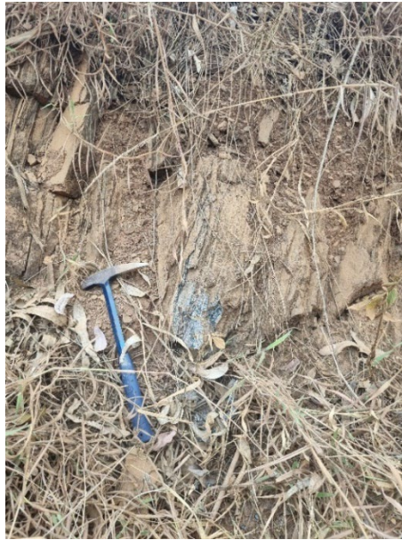
Figure 16 – Outcrop on the edge of the vicinal road. Poor, medium to coarse grained and friable quartz itabirite.
