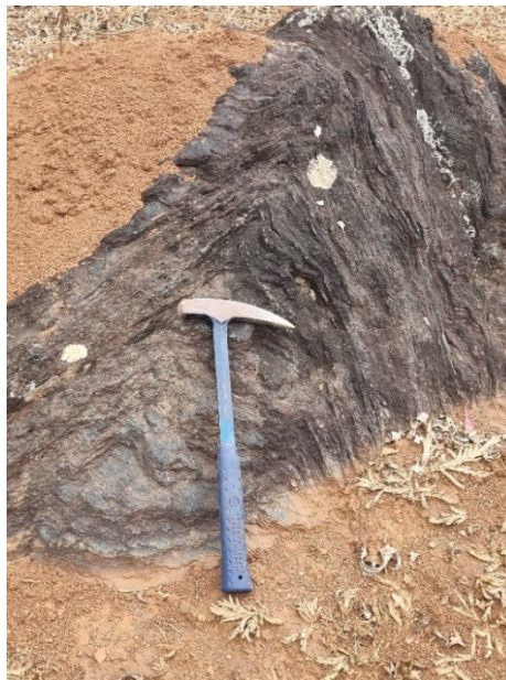
Figure 17 – Outcrop showing Boulders of quartz itabirite and tight folds.
