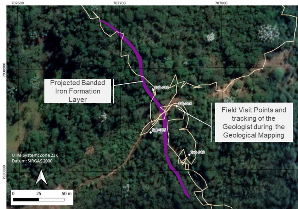
Figure 19 – Location Map of Geological points at South Eucalipto Target. In purple is shown the projection of the Iron Ore and in white the Geological Points.
