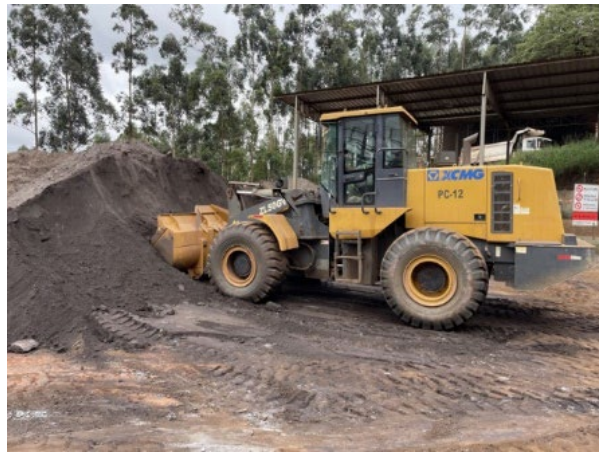
Figure 36 – Benches, stockpiles, rom pad and feed ore to crusher by front loader.
