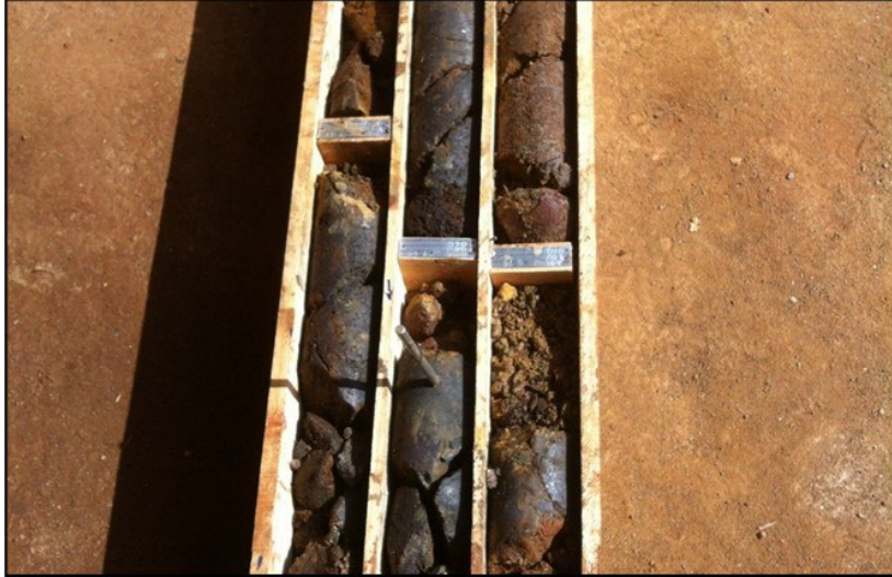
Figure 24 – Drill hole core with high grade iron mineralization intercepted at Alipio Sul Target
