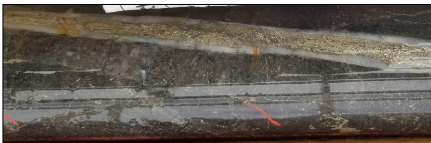
Pyrite and chalcopyrite mineralization within a B type quartz vein in potassic altered volcanics in MZ-19-01
